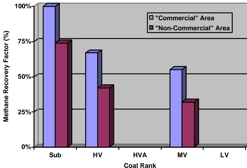
**Figure 7: Recovery Factors as in Function of Coal Rank**
