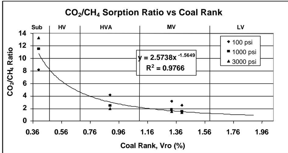
Figure 3: CO<sub>2</sub>/CH<sub>4</sub> Replacement Ratios vs. Coal Rank.
