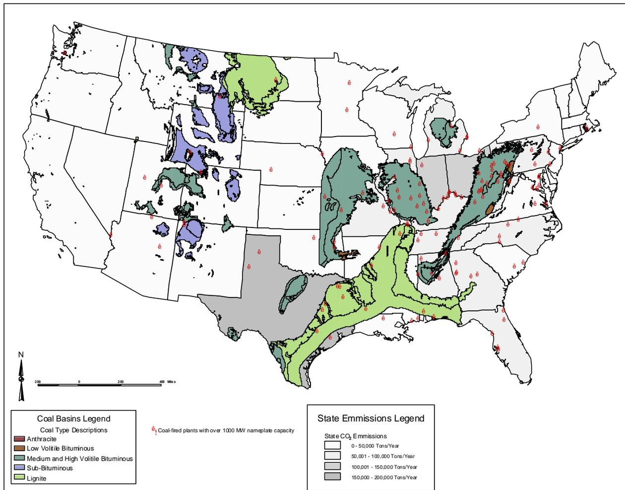
**Figure 1: Location of Major Coal Basins, Coal-Fired Power Plants, and CO<sub>2</sub> Emissions States**
