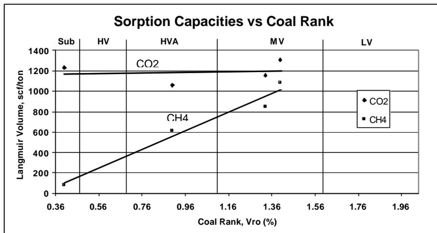
Figure 4: CO<sub>2</sub>/CH<sub>4</sub> Sorption Capacities Ratio vs Coal Rank
