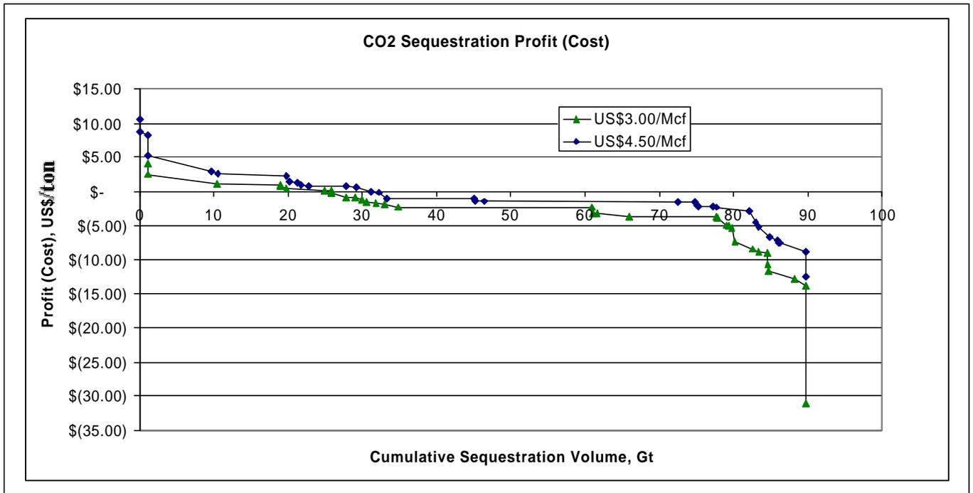
**Figure 15: Illustration of Sequestration Economics as a Function of Cumulative CO<sub>2</sub> Sequestration Capacity**
