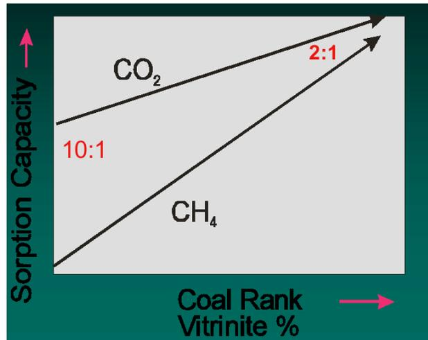
Figure 2: CO<sub>2</sub>/CH<sub>4</sub> Sorption Capacities vs. Coal Rank, from Bustin<sup>42</sup>
