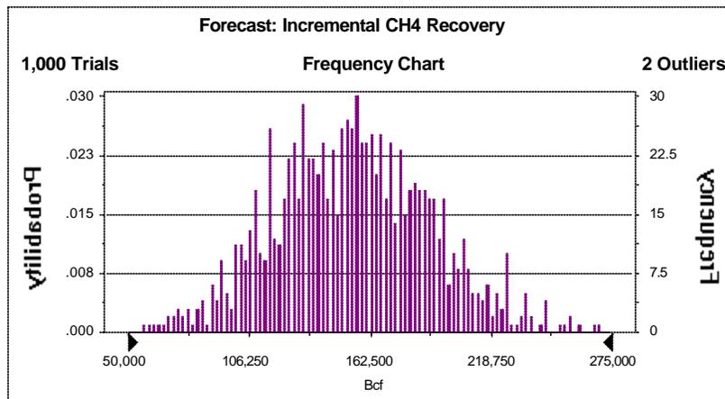
**Figure 12: Monte-Carlo Simulation Results – ECBM Potential**
