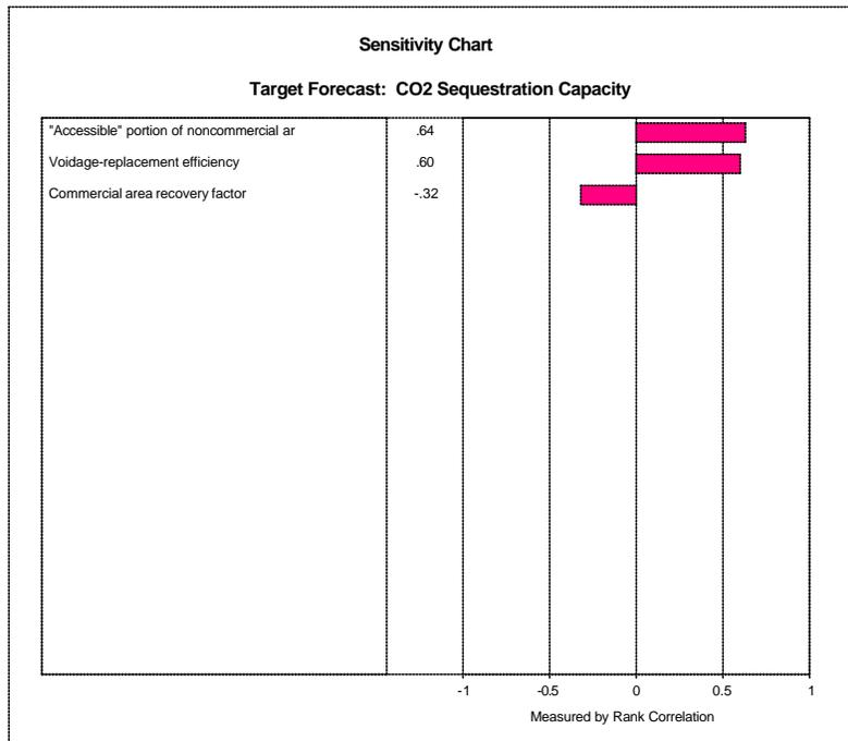
**Figure 13: Sensitivity of CO<sub>2</sub> Sequestration Capacity to Major Assumptions**
